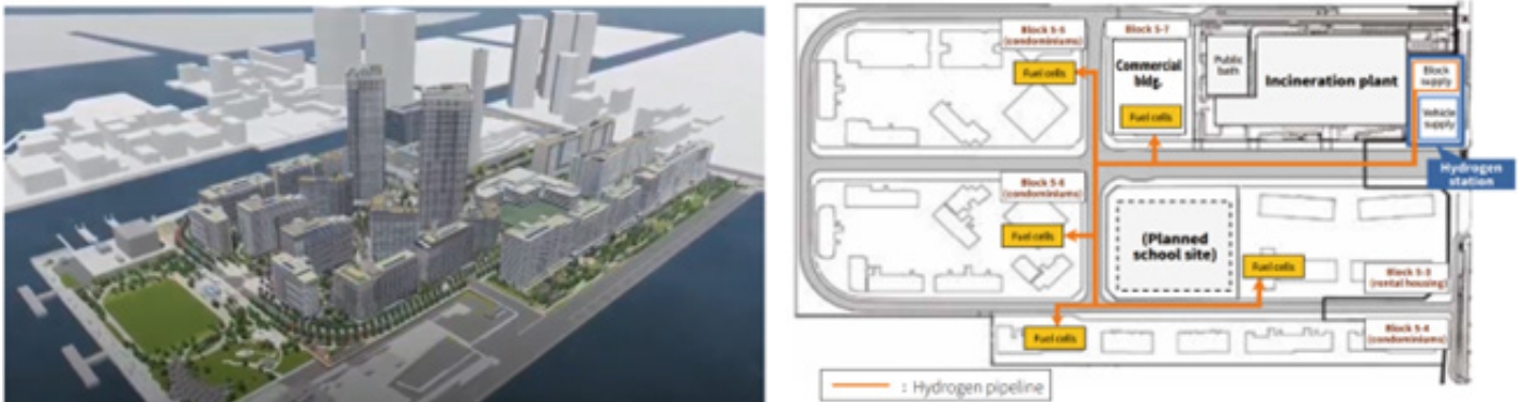
Figure 1: Harumi Flag after completion - bird's eye view and hydrogen supply conceptual schematic (Tokyo Updates, 2021)
